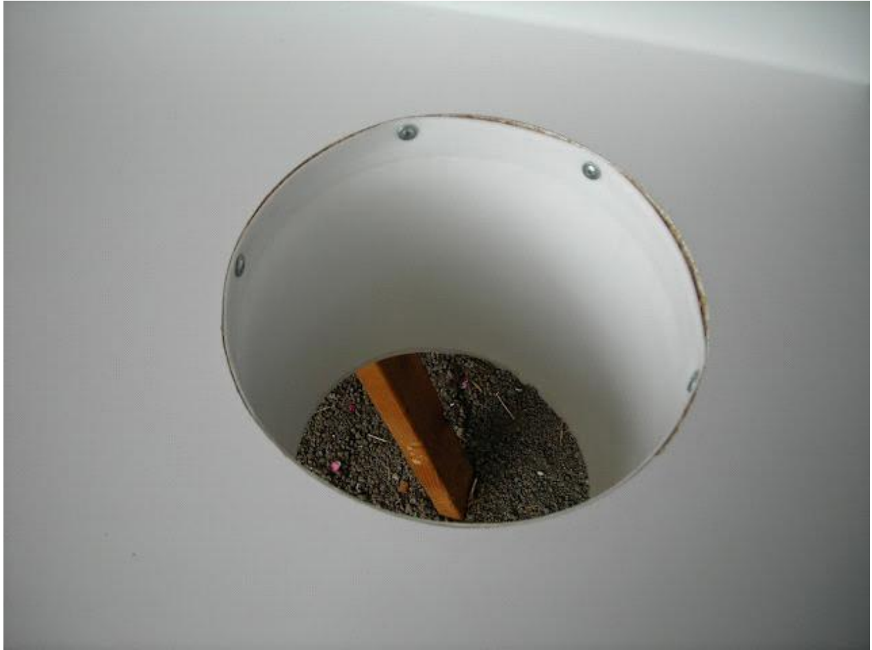
Fig. 13. Customized table used for filling up plastic bags with compost (Photo credits:fungiforum.com)
