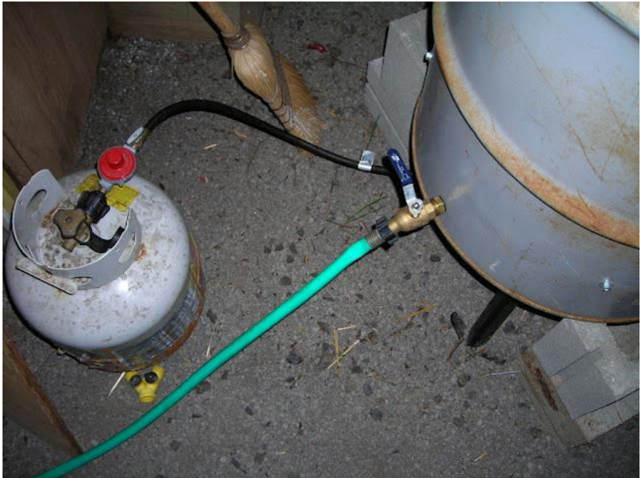
Fig. 11. Fire source and metal barrel needed in the substrate pasteurization process
